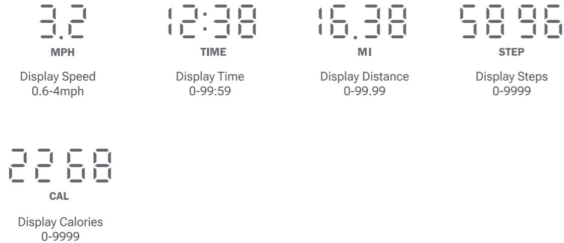
**Tips:** The workout datas (Calorie; Time; Step; Distance; Speed) will be circularly displayed per 5s.
